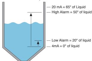
Enter all values into the LC52 in inches. The OFFSET is the corresponding 4 mA setting in inches. The SPAN is the corresponding 20 mA setting in inches. RLY1 is dedicated to the high level alarm because it is a single set point relay. RLY2A is dedicated to the low level alarm because the latch is turned off on Relay 2. Use the following values for programming the LC52-1001.
