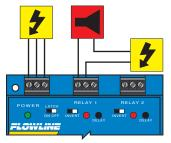
To do this, connect the hot lead of the alarm to the NC side of the relay terminal of the LC52. If
