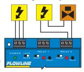
**NOTE:** If the device's load exceeds the rating of the controller's relay, a stepper relay of higher capacity must be used as part of the system design.
